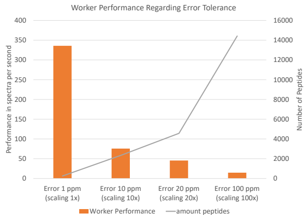
Figure 7: Average worker performance in spectra per second by increasing the error tolerance for the peptide query in MStream.
