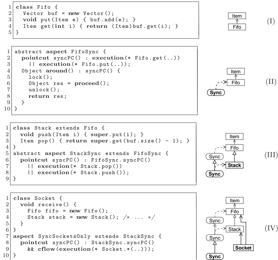
Fig. 1. A SWR example using aspects (AspectJ code).
